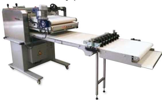
Moulder FTZ-600S-DR DYNAMIC with cutting system for small bread.
